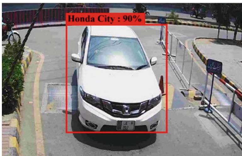
Fig. 8 Prediction on frame for detection and classification
