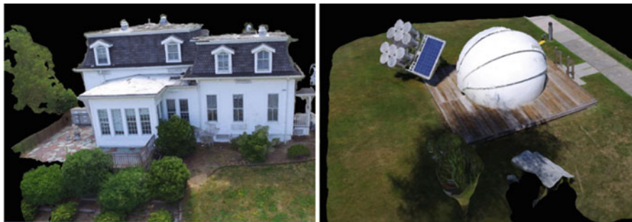
Fig. 7 Example of 3D-reconstructed image from 2D drone images [19]
