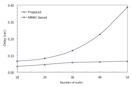
Figure 3. Channel access delay for different node densities.
