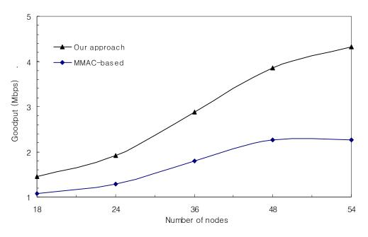
Figure 5. Goodput comparison in different node densities.
