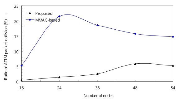
Figure 4. Ratio of ATIM packets collision in various node densities.
