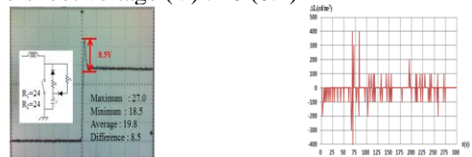
(a) Electrical characteristic (b) Optical characteristic Fig. 19 Electrical and optical characteristics of proposed circuit by overshoot
