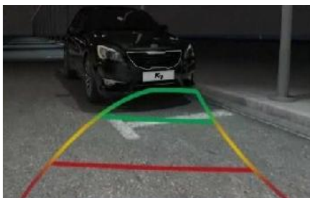
Figure 2. Parking Assist System using camera
