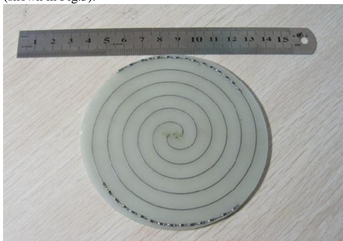
Figure 3. Partly resistive loaded spiral antenna
