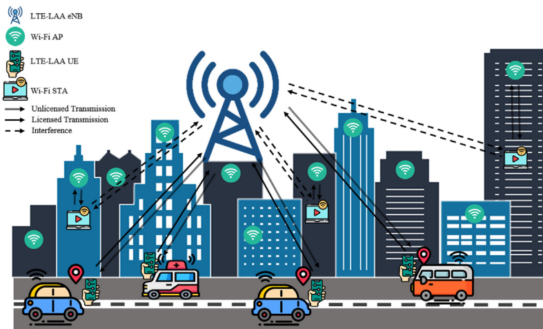
Fig. 1. LTE-LAA and Wi-Fi coexistence deployment and interference scenario in the IoT system.
