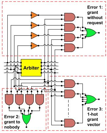
Figure 6. Fault Detection Circuitry for Arbiter.
