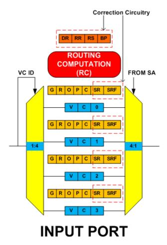
Figure 3. Fault-Tolerant RC Unit Design.
