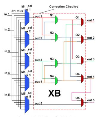
Figure 8. Fault-Tolerant XB Unit Design.
