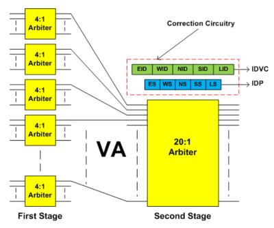
Figure 5. Fault-Tolerant VA Unit Design.
