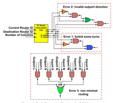
**Figure 4.** Fault Detection Circuitry for RC Unit.
