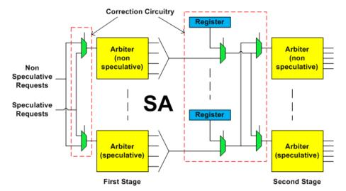
Figure 7. Fault-Tolerant SA Unit Design.
