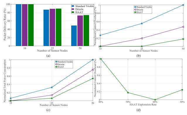
Fig. 1: (a) PDR; (b) Control overhead (%); (c) power consumption (Normalized); (d) Exploration rates and their effect on HAAT performance
